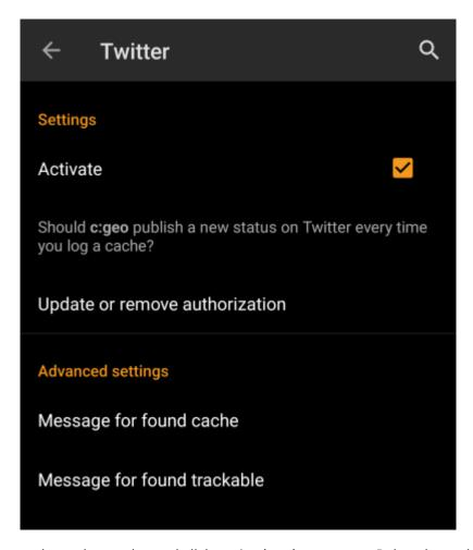
To authorize to Twitter activate the service and click on Authorize c:geo. Below the authorization buttons you can modify the templates which are used to post a message on Twitter. This template uses the same Placeholder templates as in your logging signature.
