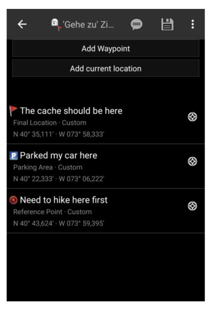
Just enter the coordinates by clicking on the coordinate section to open the input dialog. If you want to perform a waypoint projection from this position you can optionally enter the bearing and distance below.
