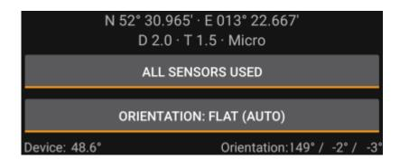
The top section of the compass screen shows the target coordinates and the D/T-rating and size information of the cache.
