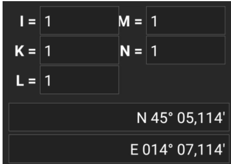
In some cases the result field still stays gray because the coordinate parser could not interpret the initial coordinate input correctly. In the screenshot below there is a misplaced SPACE character between two digits of the same group which confuses the coordinate parser.
